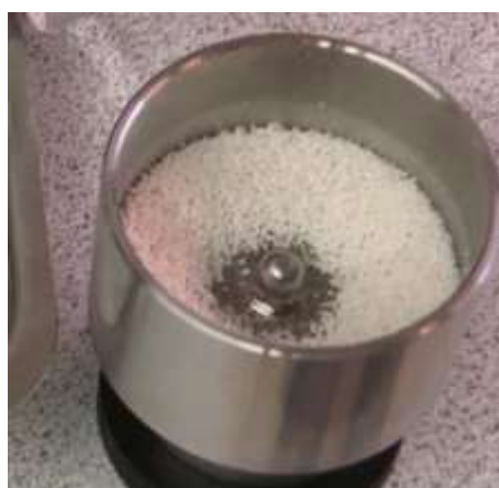
Fig 3 Formation of Pellets using spheronizer
